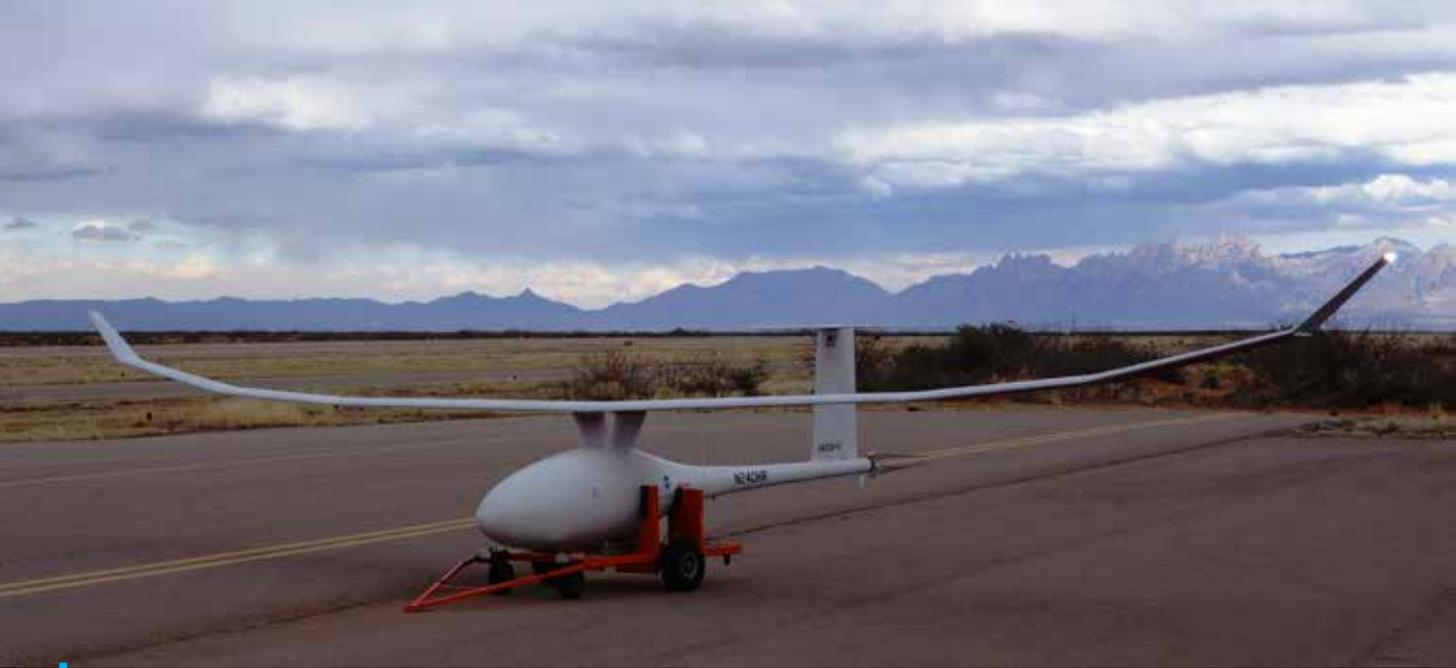
**+** The VA-001 uses a proprietary blend of solar power and fuel to maintain its endurance.
